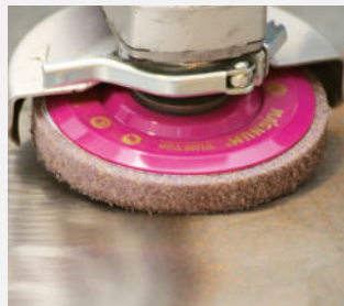
Steel: Fine grinding, deburring, rust removal
