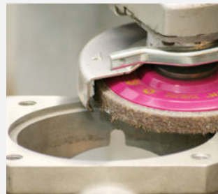
Aluminium: Cleaning, fine grinding
